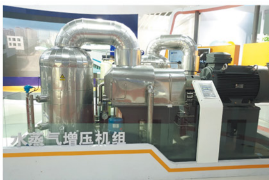
Water vapor compressor unit
